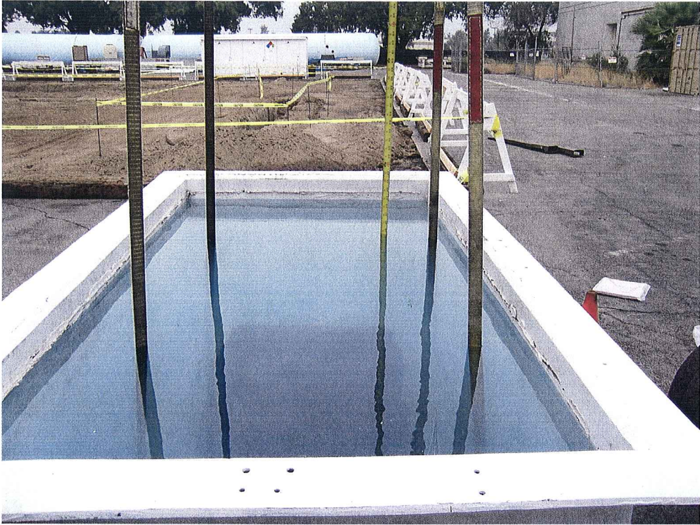
Photograph 5 Immersion Test Setup
