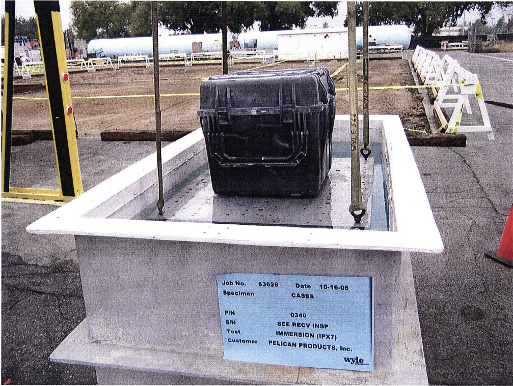
Photograph 4 Immersion Test Setup
