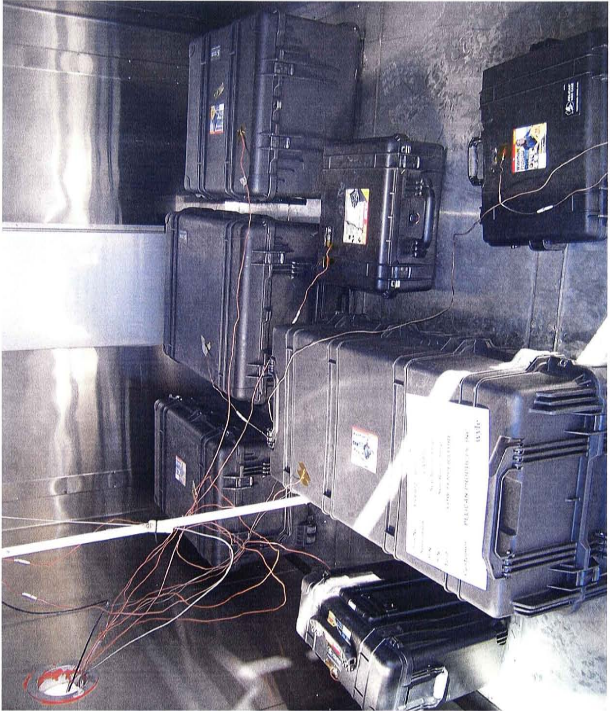
Photograph 5 Low Temperature Test Setup
